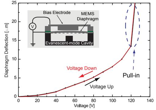
Fig. 5. Measured deflection of the MEMS actuator with bias voltage tuning up and down [23]. No hysteresis is observed.
