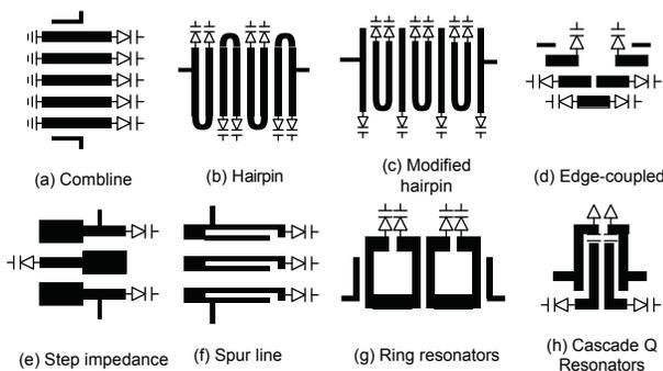
Fig. 2. Planar tunable filter architectures (adapted from [5]): (a) Combine; (b) Hairpin; (c) Modified Hairpin; (d) Edge-coupled; (e) Step impedance; (f) Spur line; (g) Ring resonators; (h) Cascade Q resonators. The “diode” symbol represents a general tuning element, which can be implemented with a variety of techniques.
