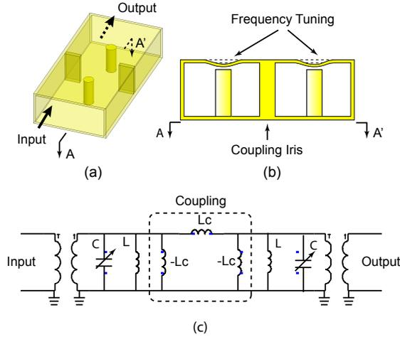
Fig. 3. Tunable evanescent-mode cavity filter. (a) Capacitive post loaded evanescent-mode waveguide filter; (b) Frequency tuning; (c) Equivalent circuit.
