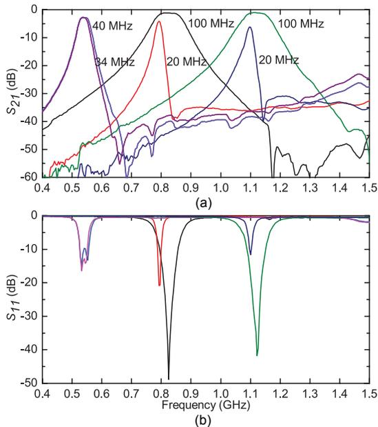
Fig. 7. Measured (a)  $S_{21}$  and (b)  $S_{11}$  showing the maximum and minimum bandwidths at selected frequencies. The filter can continuously tune center frequency and BW [26].
