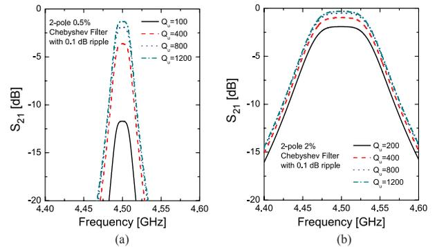
Fig. 1. Simulated  $S_{21}$  of two Chebyshev bandpass filters with different  $Q_u$ . It is evident that high- $Q_u$  resonators are necessary achieve low  $IL$ .
