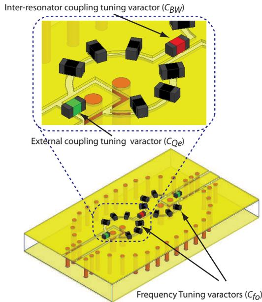
Fig. 6. Proposed substrate-integrated 3-D coaxial cavity two-pole filter and close up of top surface showing the various lumped components [26].
