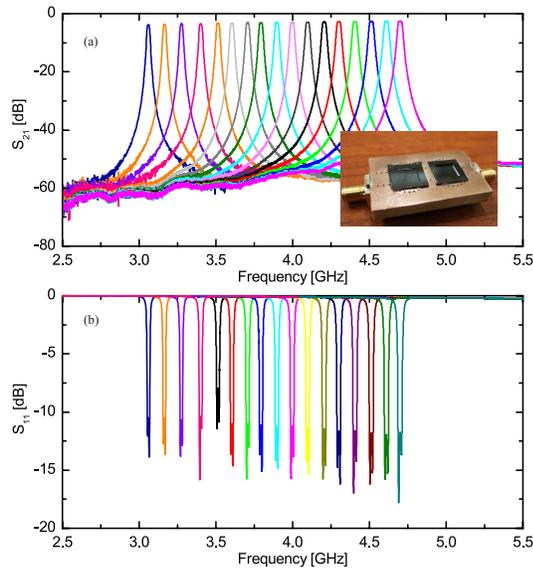
Fig. 4. Measured S-parameters of the 2-pole evanescent-mode tunable filter (a)  $S_{21}$  and (b)  $S_{11}$  [23]. The inset shows a picture of the measured device.
