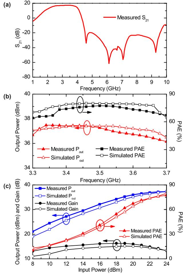
Fig. 7. Measured and simulated PA performances.
