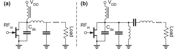
Fig. 1. (a) Lowpass filter based class-F power amplifier. (b) Bandpass filter based class-F power amplifier.
