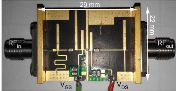
Fig. 6. Picture of the fabricated PA.
