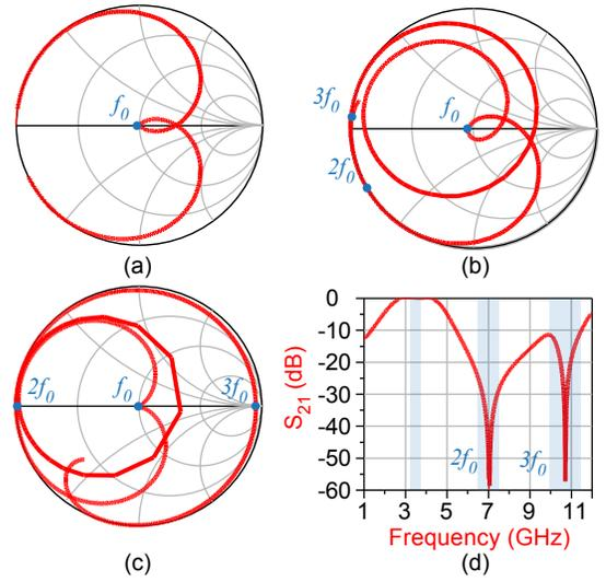
Fig. 4. (a)  $S_{11}$  of lumped component network. (b)  $S_{11}$  of distributed elements network without optimization. (c)  $S_{11}$  of optimized distributed elements network
