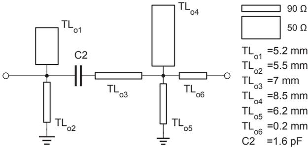
Fig. 3. Output matching network after the optimization.
