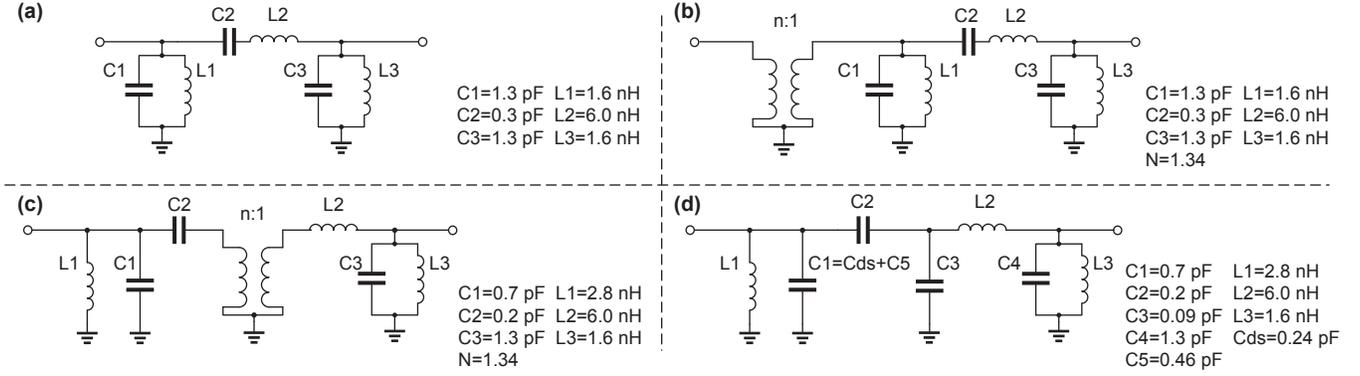
Fig. 2. (a) Three stages synthesized chebyshev bandpass filter. (b) Synthesized chebyshev bandpass filter with left port impedance of  $90 \Omega$ . (c) Move transformer to the middle part of the synthesized chebyshev bandpass filter. (d) Synthesized chebyshev bandpass filter after Norton's transform.
