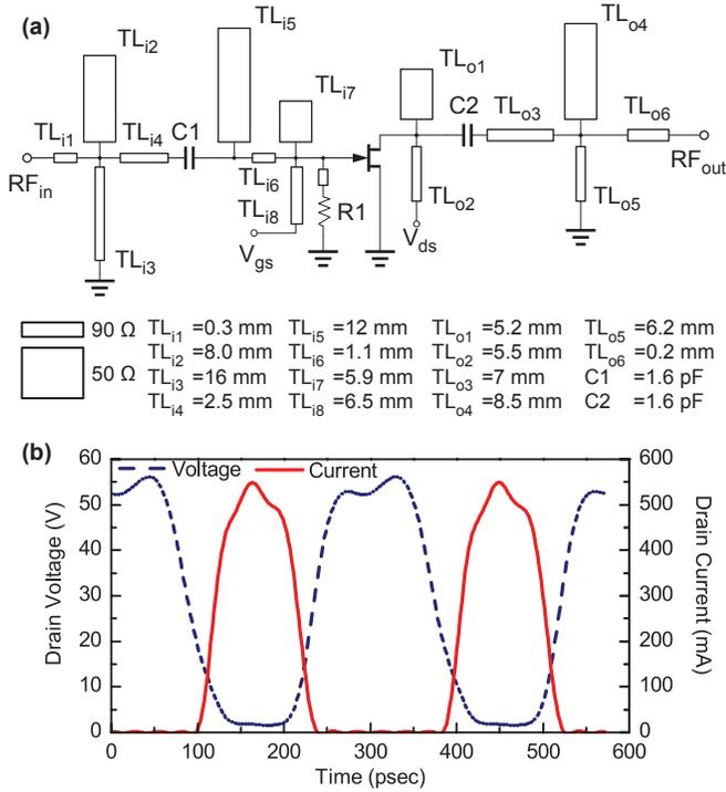
Fig. 5. (a) Optimized schematic of the complete PA; (b) Simulated current and voltage waveforms at the transistor current source.
