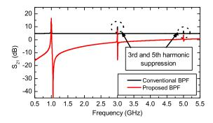
Fig. 6. The proposed filter shows both third and fifth harmonic suppression compared with all pole bandpass filter.
