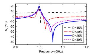
Fig. 7. The transfer function of the filter with duty cycle variations
