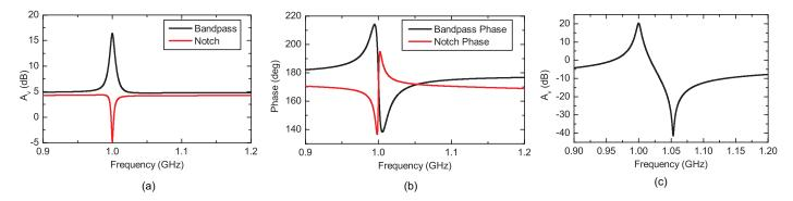
Fig. 2. (a) Magnitude response of bandpass and notch filter (b) Phase response of bandpass and notch filter (c) The overall filter response including DDA gain ( $\sim 5$  dB).
