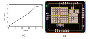
Fig. 10. (a) Simulated out-of-band IIP3 of the filter for different offset frequencies from center frequency of the filter. ( $f_{lo}$ =1 GHz) (b) Chip layout of the proposed filter.
