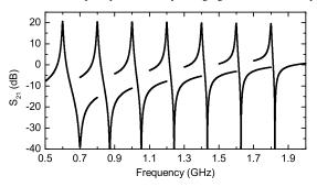
Fig. 9. The simulated transfer function of the filter shown at every 200 MHz over the frequency range from 0.6 GHz to 1.8 GHz.
