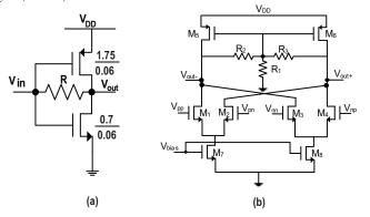
Fig. 3. (a) The unit  $G_{\rm m}$  cell that is used with different scaling factors (b) The differential difference amplifier
