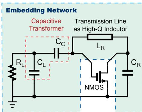
Fig. 1. Schematic of the proposed 213-GHz oscillator
