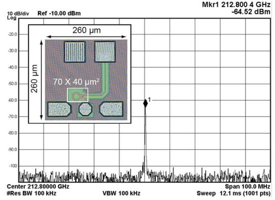
Fig. 7. Screen capture of the spectrum measurement of the fabricated oscillator. Inset: Die photograph.
