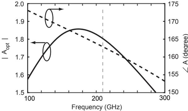
Fig. 4. Simulated optimum complex voltage gain  $A_{opt}$ .
