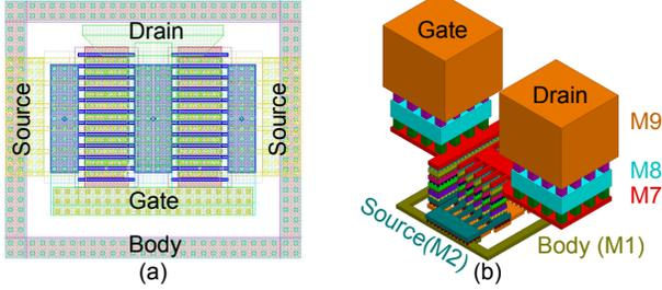
Fig. 3. (a) Layout of the 20- $\mu\text{m}$  NMOS transistor (b) Interconnect setup used for connecting to the transistor.
