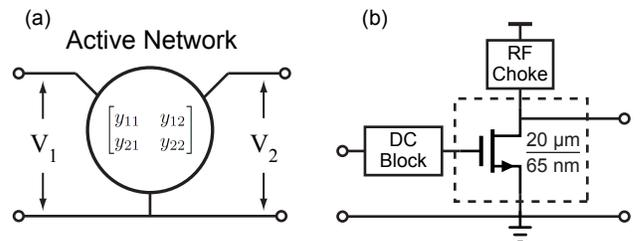
Fig. 2. (a) A general nonlinear active two-port network. (b) Two-port simulation setup for extracting the large-signal Y-parameters of the NMOS transistor.
