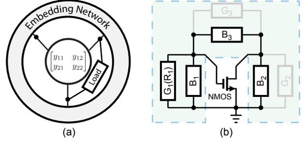
Fig. 5. (a) A conceptual representation of the Y-oscillator model. (b) Initial oscillator topology for optimal output power.
