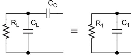
Fig. 6. (a) Capacitive transformer (b) Equivalent circuit of the transformer
