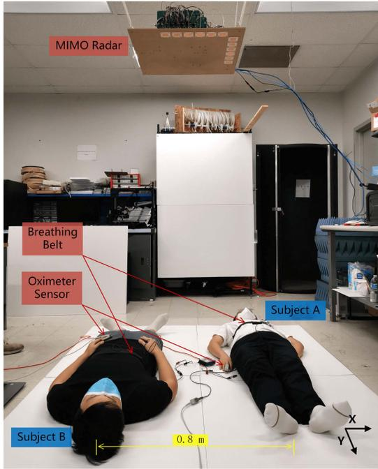
Fig. 14. Setup of Experiment 3: the multitarget vital signs measurement of lying people.
