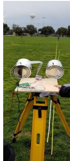
Fig 17. Completed Radar System
