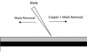
Figure 6, Scraping direction for material removal
