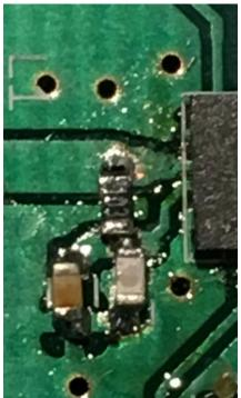
Figure 7, RF trace shunt elements
