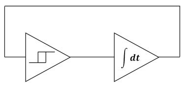
Figure 1, block diagram for triangle wave generator
