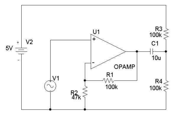
Figure 4, triangle wave amplifier
