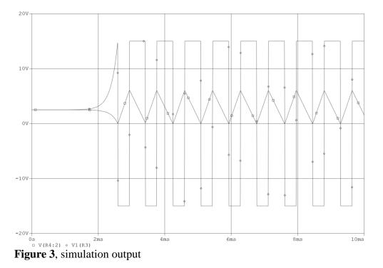
The sync output comes from the output of the Schmitt trigger, the triangle wave comes from the output of the integrator. If a quad op-amp is used, such as the TL974, the outputs can be sampled without perturbing the feedback loop using non-inverting amplifiers or voltage buffer configurations due to their very high input impedance. The biasing voltages can be most easily accomplished using a voltage divider with a trimmer so it can be tuned as needed to eliminate the
