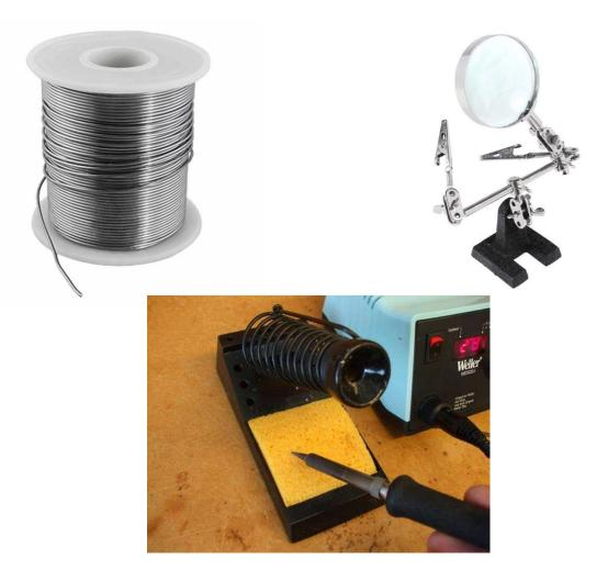
Figure 1. Images of Typical Solder Wire, PCB Holder and Hot Iron
