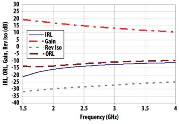
Figure 3. Gain performance depending on frequency
