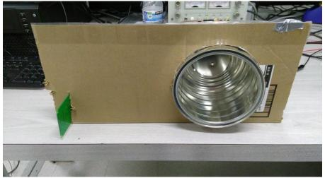
Figure 4. Final Antenna configuration
