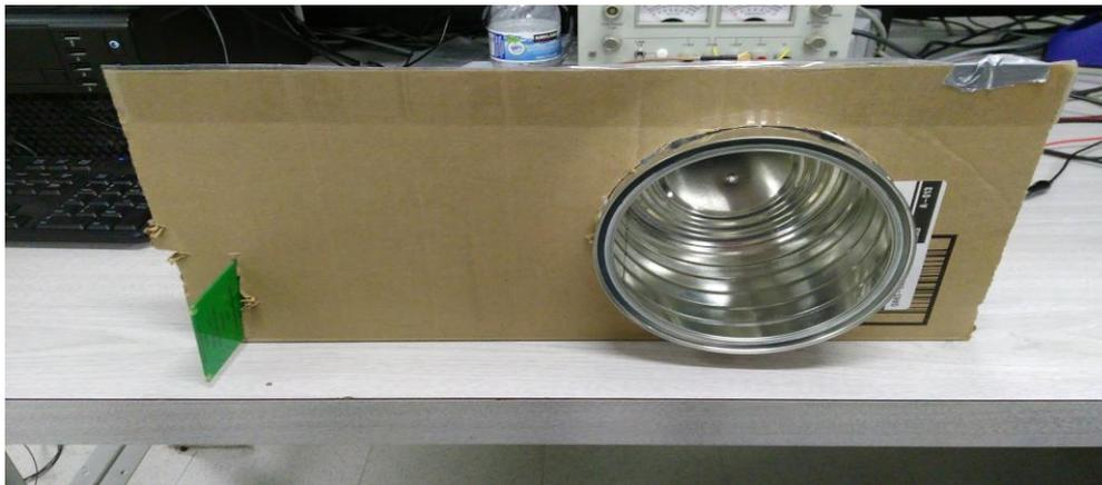
It did not make too much of a difference between having the Yagi antenna on receive and cantenna on transmit or vice versa, just the combination of the Yagi antenna and the cantenna produced the best results. Because of this, my personal recommendation is to purchase the Yagi antenna but due to its fragility, purchasing two would be beneficial as the soldering can come loose during the competition and having a backup is always a good idea.
