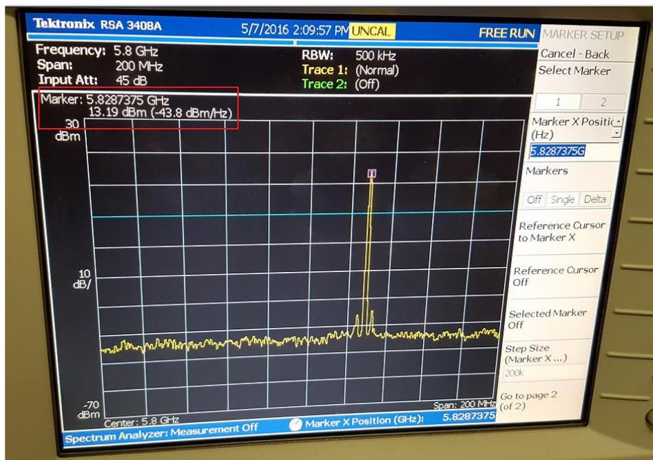
NOTE: a 3 dB attenuator was connected to the output port of the RF board to help prevent overloads.
