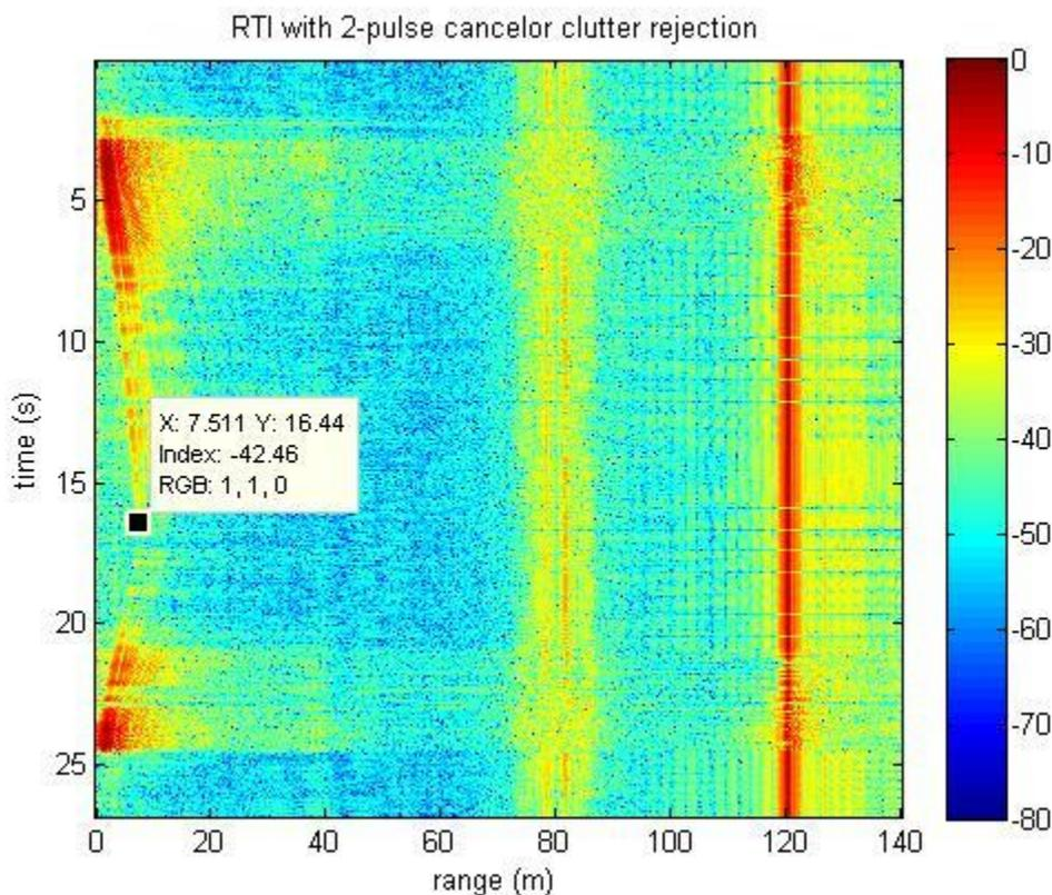
The plot shows that the radar detected the sheet moving away from the antennas and coming back, indicating that the radar can detect objects at least 7 meters away. The range intensity at the 80 meter and 120-meter range were the result of signals reflecting off the objects inside the room.
