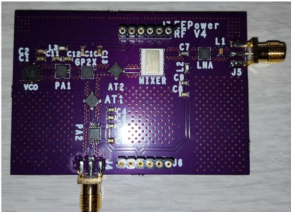
The microstrip line widths connecting each of the RF components had to be matched to 50 Ohms, so ADS LineCalc was used to compute the necessary transmission line width, as shown in figure 17. The parameters for the substrate are summarized below.
