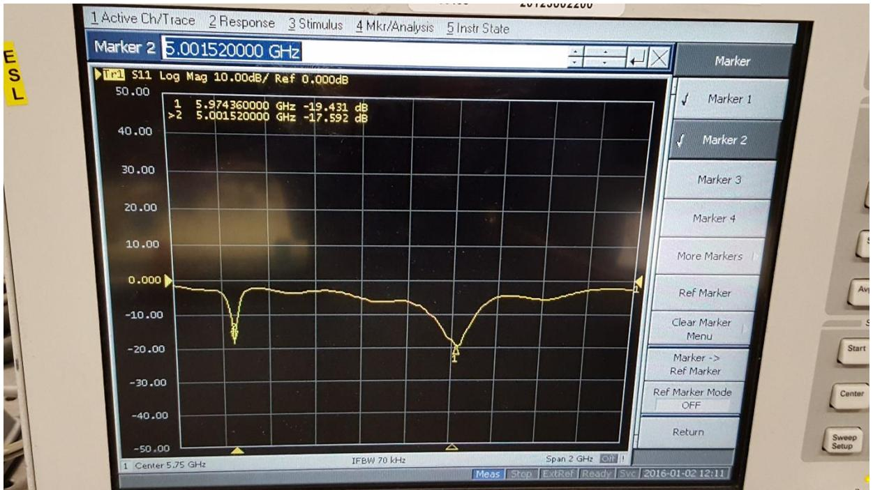
Figure 24 Antenna 2 Bandwidth
