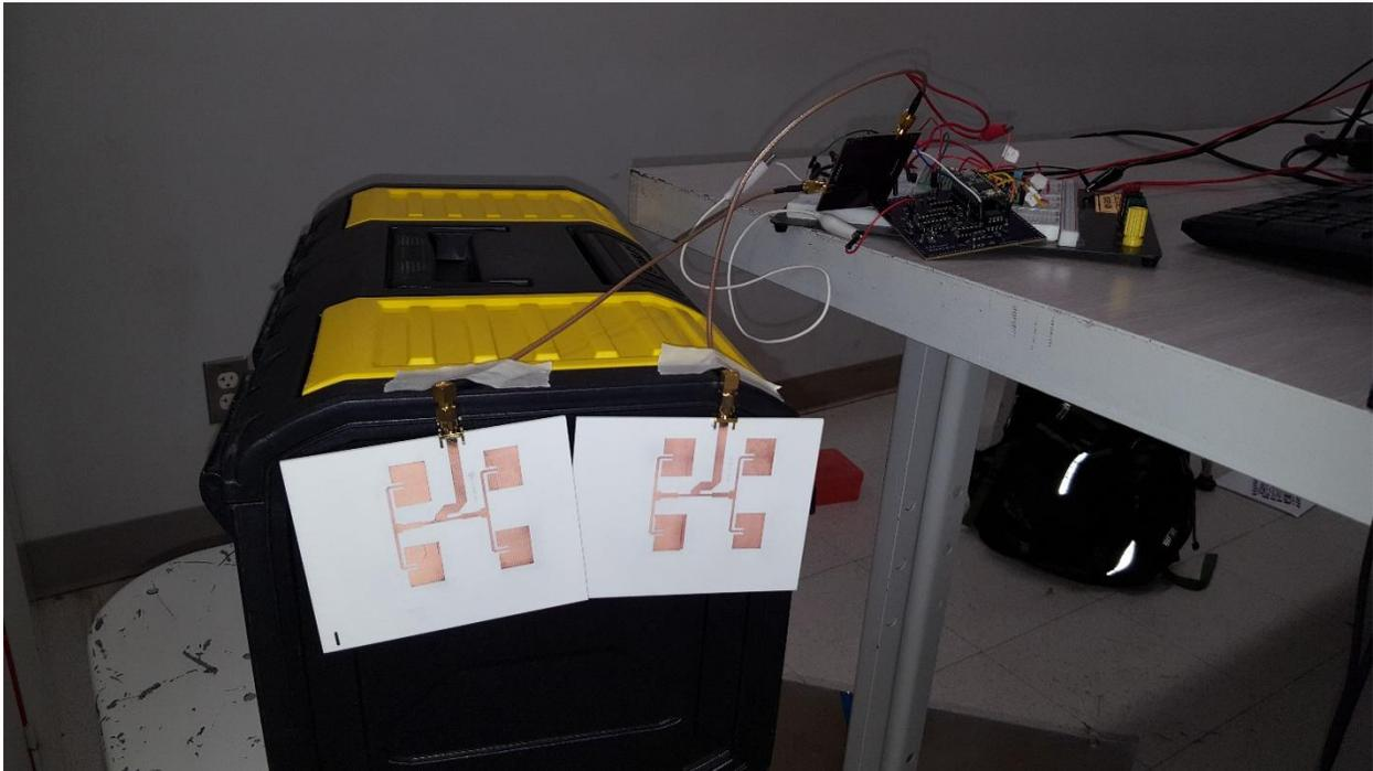
The measurement began with the aluminum sheet less than 6 inches away from the antennas. When the data collection started, the sheet was moved slowly away from the antennas until it was approximately 20 feet away, and then walked slowly back toward the antennas.
