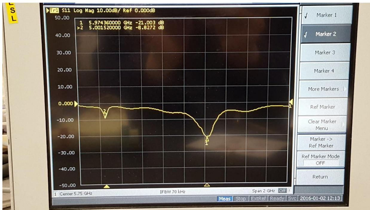
Figure 22 Antenna 1 Bandwidth
